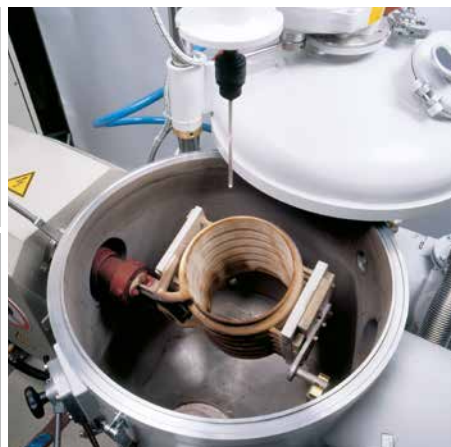
◀ Temperature measurement with thermocouple and reusable protection tube
