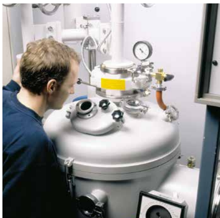
◀ Observation of vacuum induction melting and casting process via sight glass
