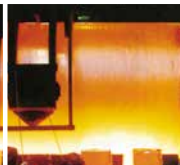
165 ton ESR ingot, 2300 mm diameter x 5000 mm long.
