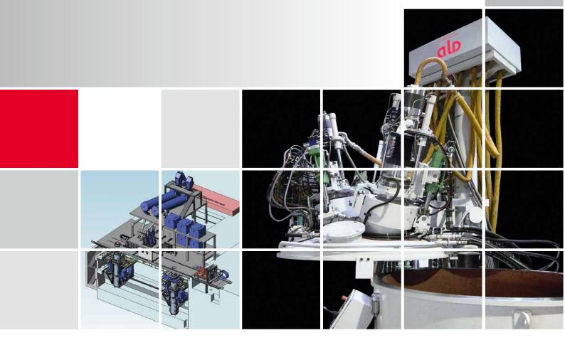
For melting and remelting of Titanium-Alloys, e.g. Titanium Aluminides, containing larger amounts of alloying elements with high vapor pressure that would evaporate under deep vacuum, the plasma arc melting process is the first choice.
