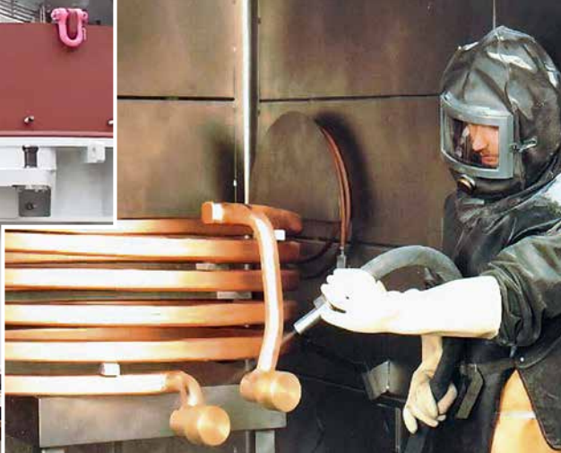
Sand blasting for gentle surface treatment
