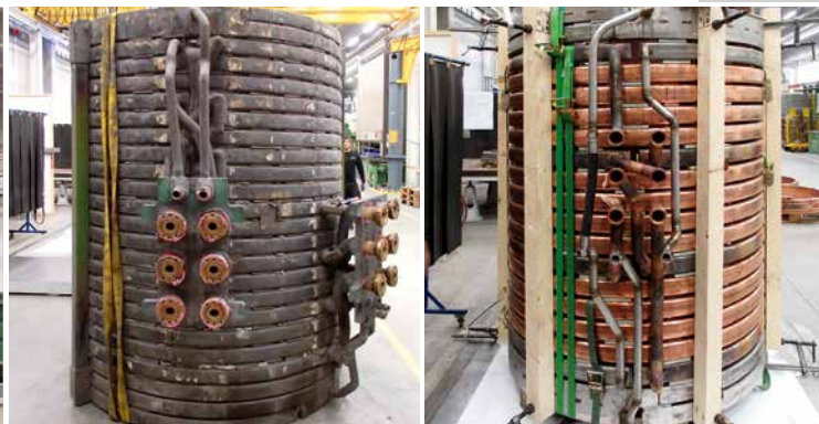
An induction coil before and after reconditioning
