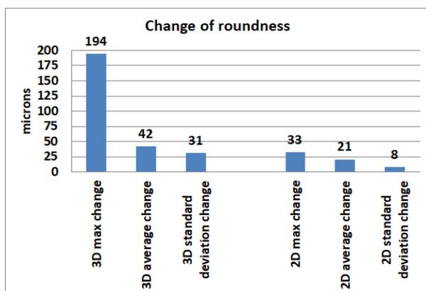
Fig. 5: Change of roundness during LPC-treatment of Final Drive Ring gears; comparison between 3D - treatment and 2D-treatment
