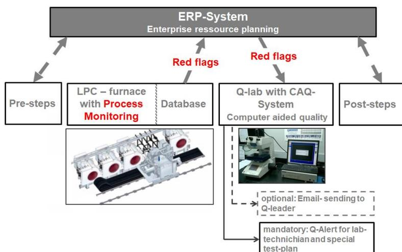
Fig. 8: Digital architecture: Process Monitoring is digitally embedded into the ERP-System and the Q-Lab
