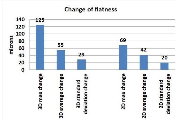
Fig. 4: Change of flatness during LPC-heattreatment of Final Drive Ring gears; comparison between 3D - treatment and 2D-treatment
