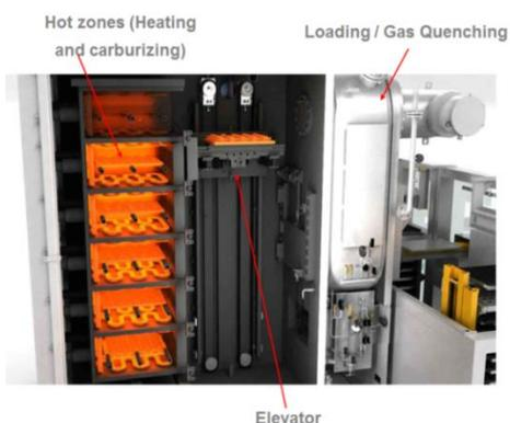
Fig. 2: Heat treat system for 2D-treatment; schematic view into the system
