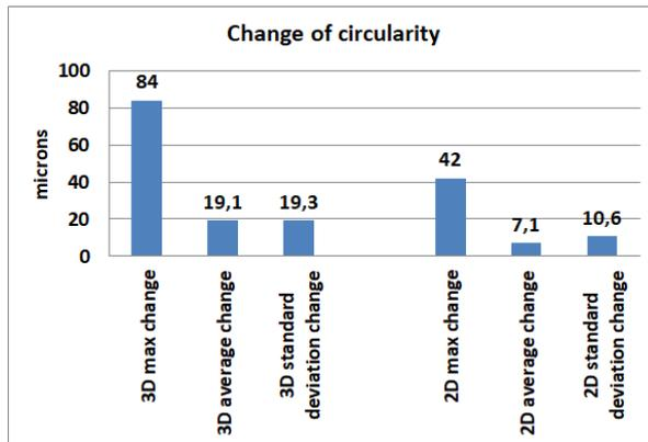
Fig. 7: Change of circularity during LPC-treatment of "Reaction Internal gear Type B"; comparison between 3D - treatment and 2D-treatment
