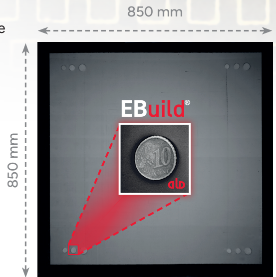
in-situ electron image of build area
