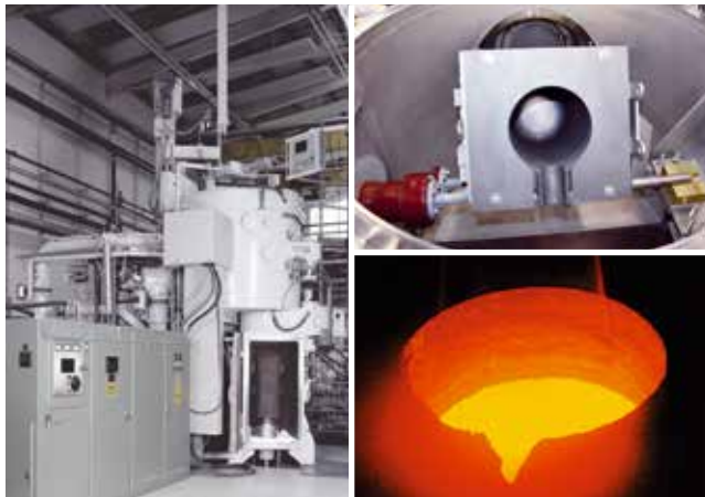
VIM70 VMC Furnace with separate Vertical Mold Chamber for ferrous and non-ferrous alloys (in combination with mold treatment directional solidification is possible)
