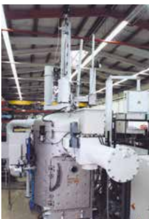
VIM50 VIM furnace with tundish heater and oxygen resp. inert gas blowing device for research and development
